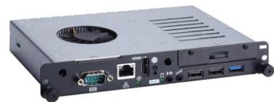
This smart open pluggable module is connected to OPS-compliant display via a standardized JAE TX-25 plug connector that supports HDMI, DisplayPort, UART, audio, USB 3.0 and USB 2.0 signals. The Axiomtek OPS883
